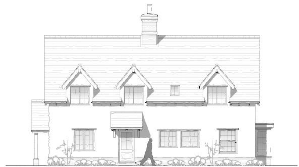
Proposed North-West Elevation Scale 1:50 @ A1 (1:100 @ A3)
